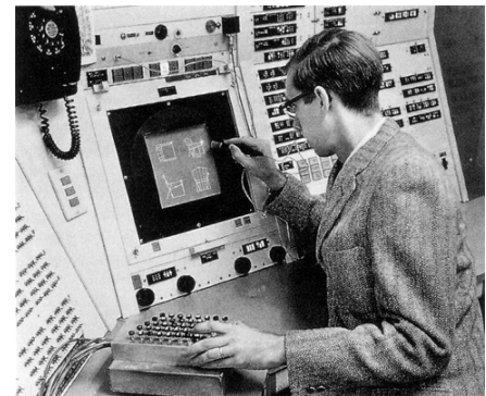
Ivan Sutherland’s Sketchpad console, 1962. Sketchpad is operated with a light pen and a command button box. The four black knobs below the screen control position and scale of the picture.
