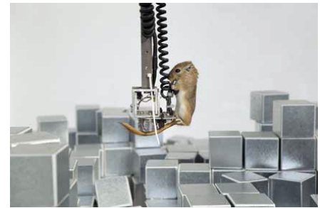
Feedback and interaction. Nicholas Negroponte's Seek from 1970. Robotic arms re-configure the arrangement of blocks after observing the gerbils' reactions to previous layouts.
